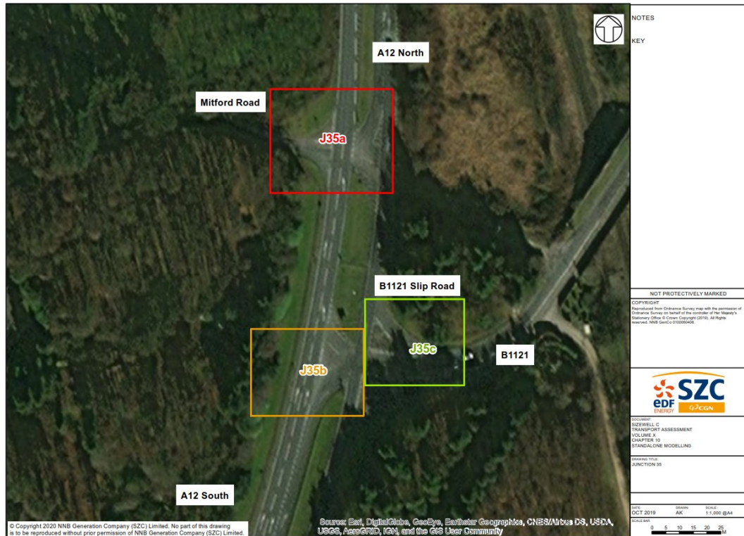
Plate 9.44 – Existing A12 / B1121 Main Road T-Junction Layout
